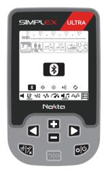
2. You can turn on or off the Bluetooth® connection using the plus (+) and minus (-) buttons. When it's off, the box will be displayed in white, when it's on, it will be in black.
