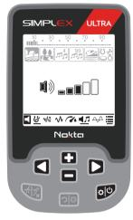
To exit the settings, press the Power & Settings button again. While in the settings menu, if no button is pressed for a while, settings will time out and the device will revert back to the main screen.
