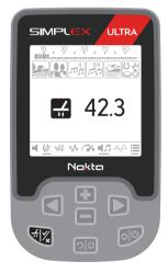
5. If you cannot ground balance, in other words, if no beep sound is produced, it means that either the ground is too conductive or not mineralized or there is a target right below the search coil. In such a case, retry ground balance at a different spot.
