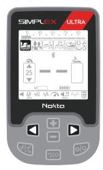
4) You can increase the sensitivity if needed. Increasing the sensitivity will offer you greater depth. However, if the surroundings or the ground cause excessive noise in the device, you need to lower the sensitivity setting.
