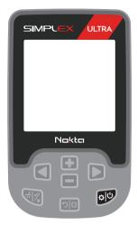
3) When the device is turned on, it will start in the 2-tone Field mode. You can change the mode based on ground conditions. For instance, if you are detecting on wet beach sand, you may want to select the Beach mode. You can find more details on search modes further in this manual.
